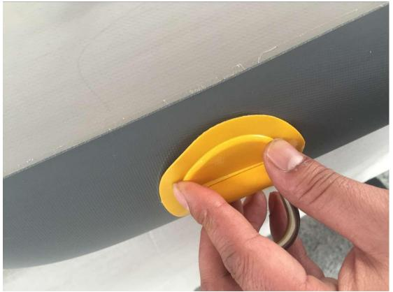
3. Glue evenly on the bottom of D-ring patch and board.
