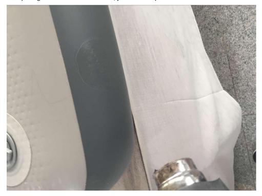
5. Heat the glued area evenly with the hot gun/hair drier, as the glue will work better after heating.
